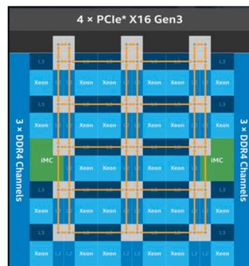
Workstations require high-bandwidth connectivity to compute, graphics, and storage resources inside the system. This generation of Intel Xeon W features 64 PCI Express lanes for massive bandwidth in and out of the processor.
