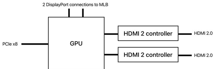
**Radeon Pro W5500X MPX Module architecture**
