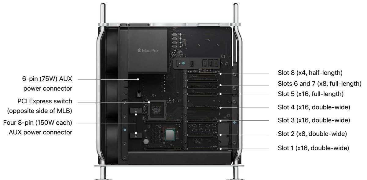
Mac Pro provides four 8-pin auxiliary (AUX) power connectors that each provide 150W of power, for a total of 600W of AUX power. This power is in addition to the 75W of power provided directly by each PCIe slot. Combined, up to four 225W graphics cards can be installed in Mac Pro, each in an x16 slot with a total power of 900W. A single 6-pin AUX power connector provides 75W of additional power for PCIe cards in slots 5, 6, and 7.
